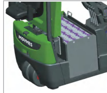
Sideway battery box
