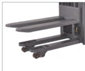
Option: Initial lifting with double-pallet function turn to P80
