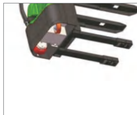
4 point design, improve the trucks stability.
